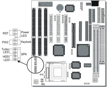
Plug the computer case's front panel devices to the corresponding connectors on the Motherboard.
